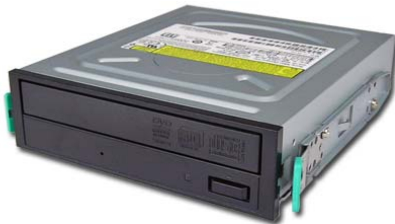
Figure 42: Attaching the Slide Rails
