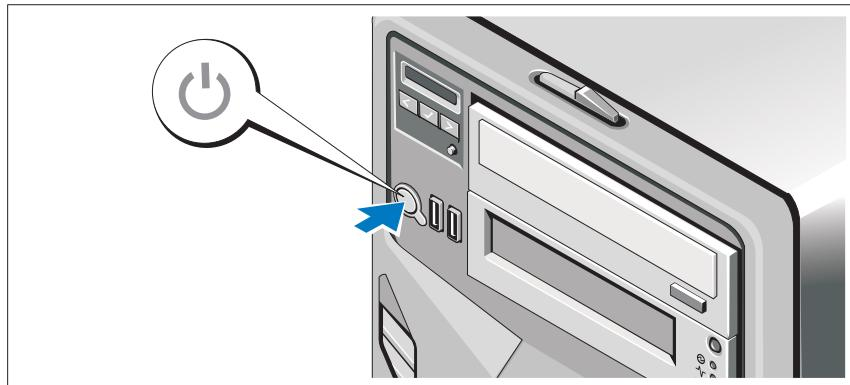
Press the power button on the system. The power indicators should light.
