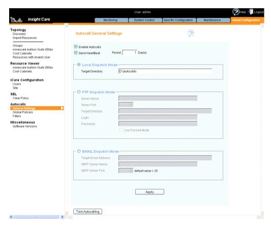
Figure 4-2. Autocall General Settings page (Autocall Enabled)
