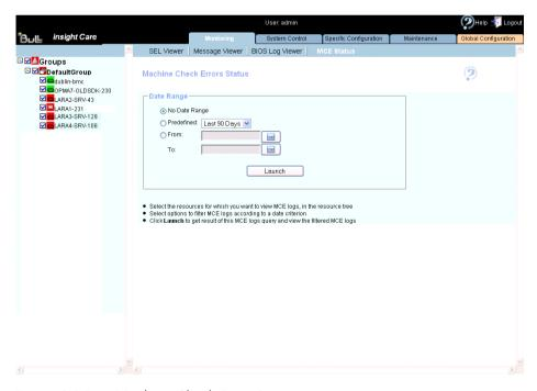
Figure 3-15. Machine Check Error Status page
