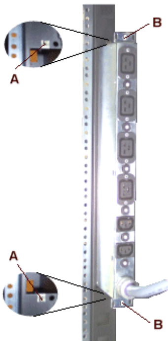
Figure 16. Installing a PDU vertically
