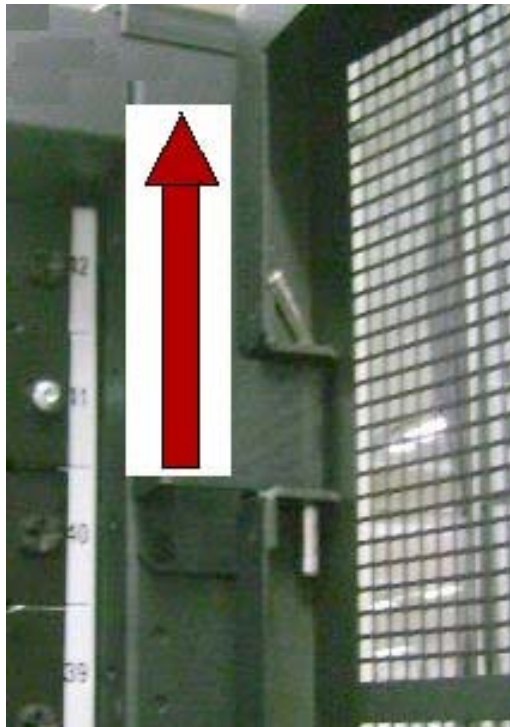
Figure 14. Removing the front door
