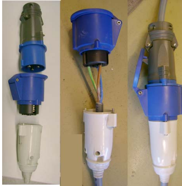
Figure 27. PDU/UPS Power socket
