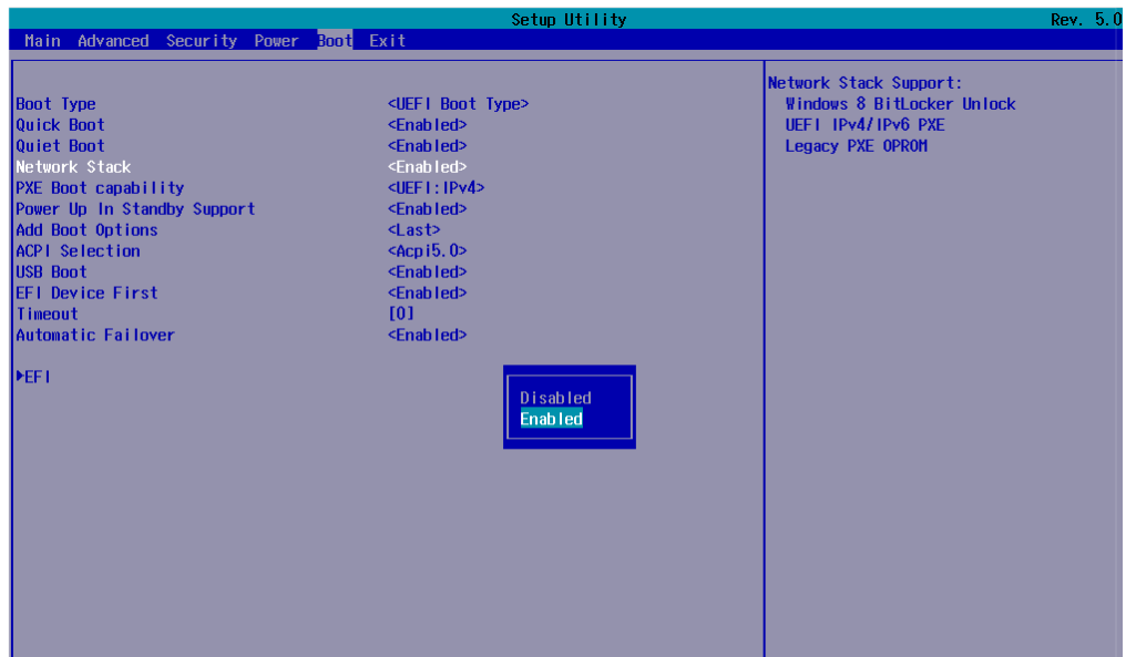
Figure 4-2. Boot configuration - Enabling Network Stack support
