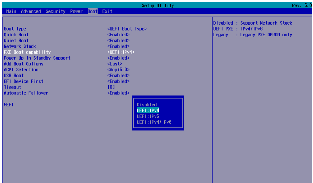
Figure 4-3. Enabling PXE Boot capability - Example
