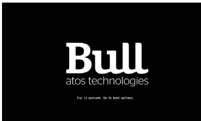
Figure 4-1. Accessing the boot options d. Press [Esc] to access the boot options.
