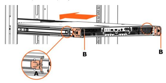
3. Tighten the captive screws to secure the server into place.
