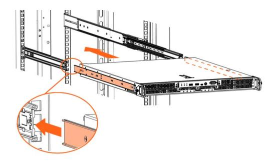
2. When the rail assemblies click, push the release latch (A) on each side to allow the server to be pushed completely into the rack.
