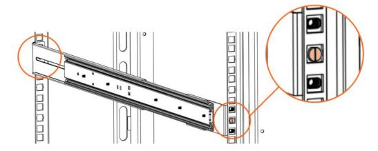
4. Secure the rail assembly into place.
