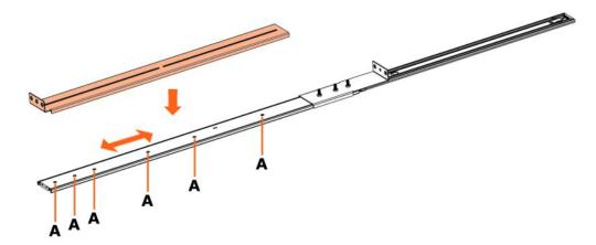
2. Adjust the rear bracket position on the outer rail to match the rack cabinet depth.
