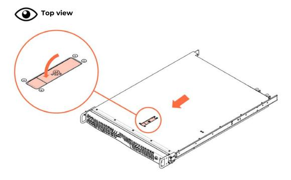
3. Tighten the captive screw to lock the cover latch.
