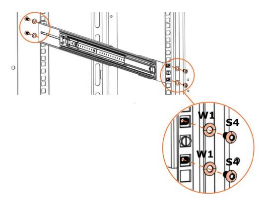
5. Tighten the rear bracket nuts.
