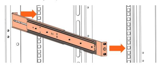
2. If necessary, adjust the length of the rail assembly by sliding the rear bracket.
