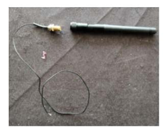
2. Remove the nut and the washer from the connector.
