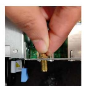
4. Install the washer and the nut onto the connector.
