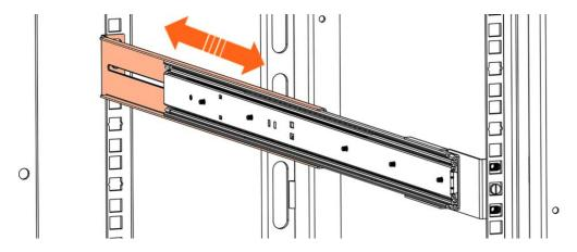
3. Position the rail assembly using the guide pins at each end.
