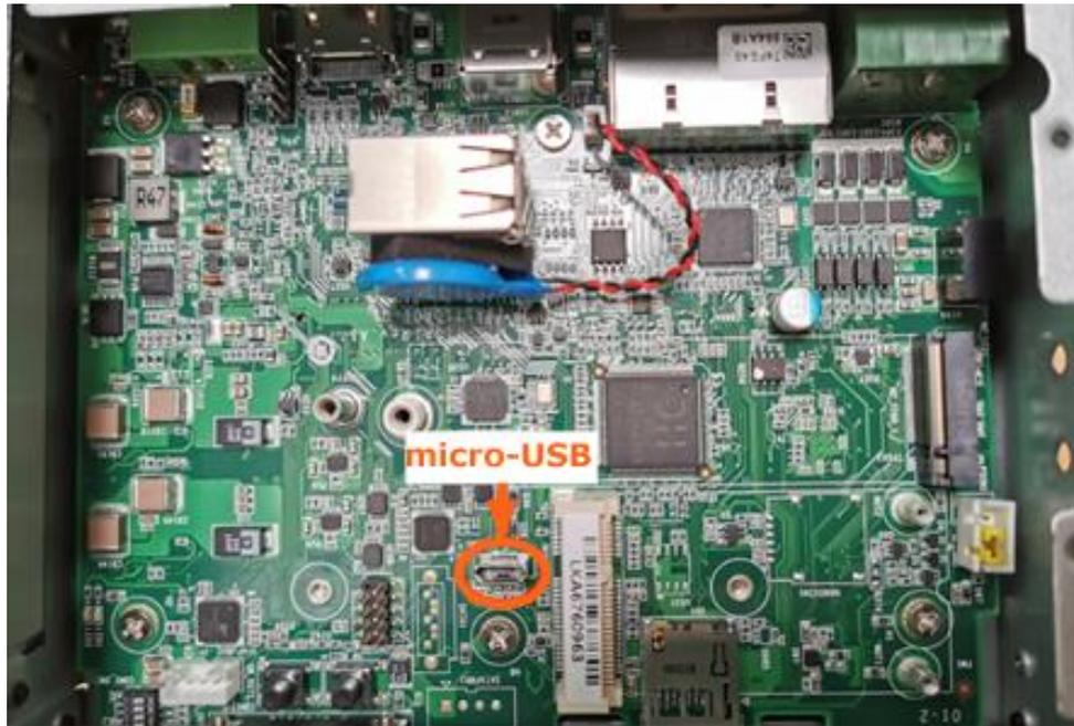
5. Connect the host system to the BullSequana Edge nano server with the USB cable supplied.
