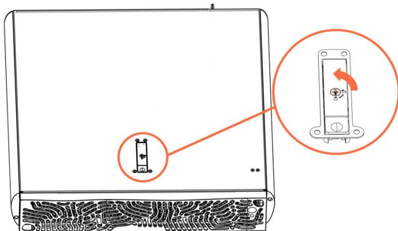
2. Push the button (A) to release the latch. The upper part (B) rises up.
