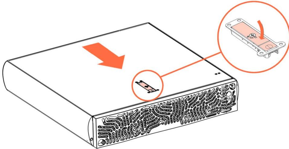
3. Tighten the captive screw to lock the cover latch.
