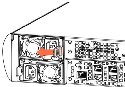
2. Take hold of the handle and remove the PSU.
