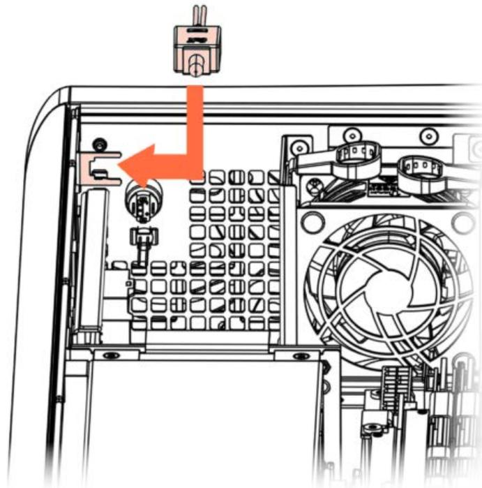
2. Connect the sensor cable to the motherboard.
