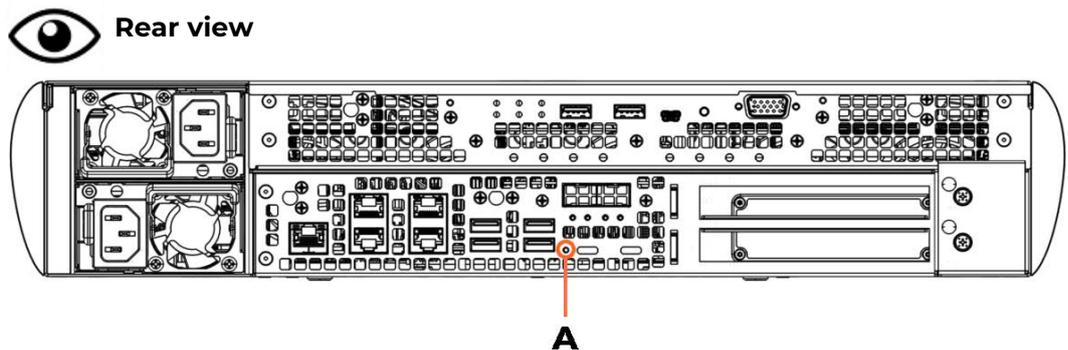
2. Push the button in using a pointed object and release.
