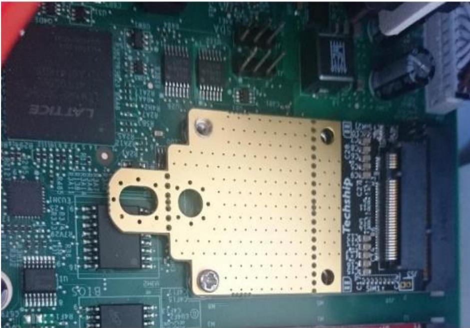
**Step 3 :** After that you can plug the M.2 card into the mPCIe M.2 slot.
