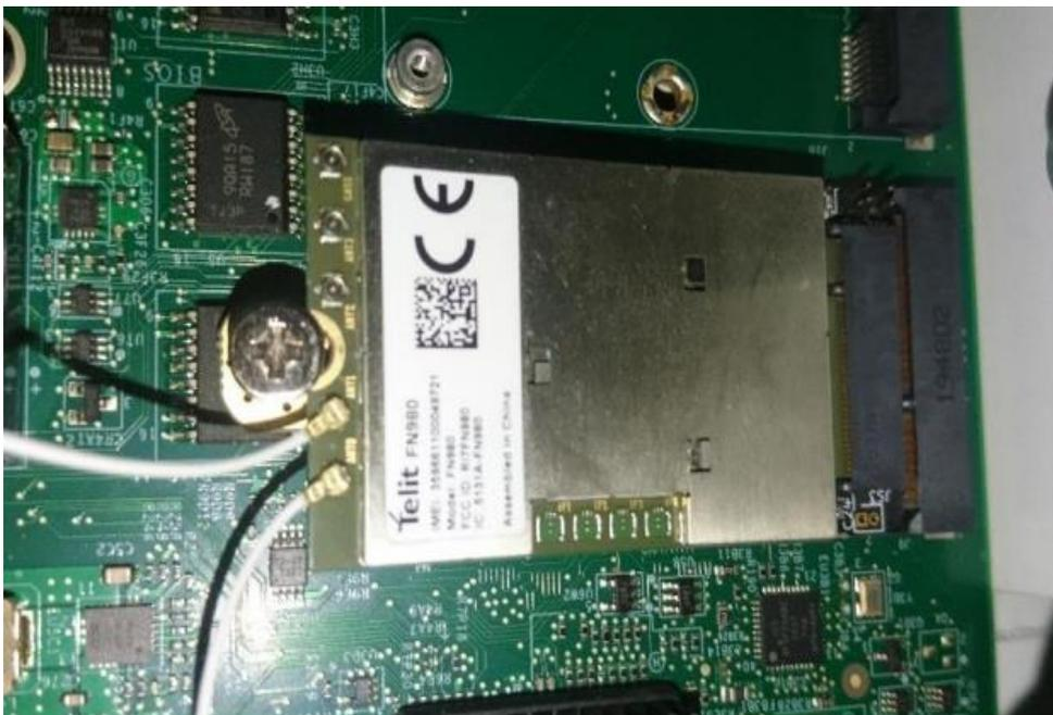
**Step 4:** To finalize the installation, you need to connect the antenna as required.
