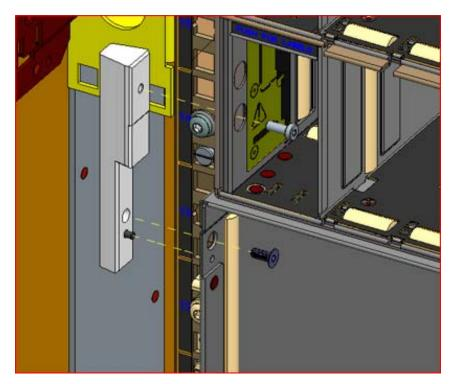
3. Install the 8-module connecting box as described in the Installation Guide
