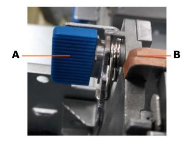
2. Press the latch (A) down to secure the HDD cage in place.
