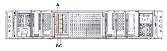
2. When the Ethernet link activity LED (C) blinks amber, run the following command.
