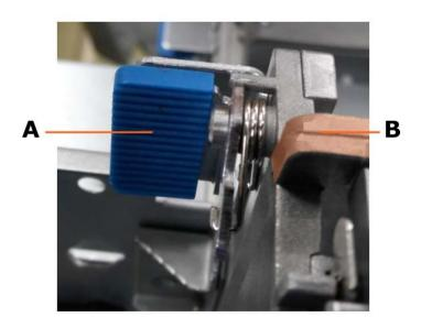
2. Press the latch (A) down to secure the HDD cage in place.
