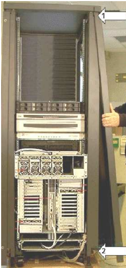
Figure 22. Refitting side covers – 36U cabinet
