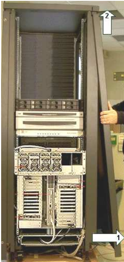
Figure 7. Removing side covers – 36U cabinet
