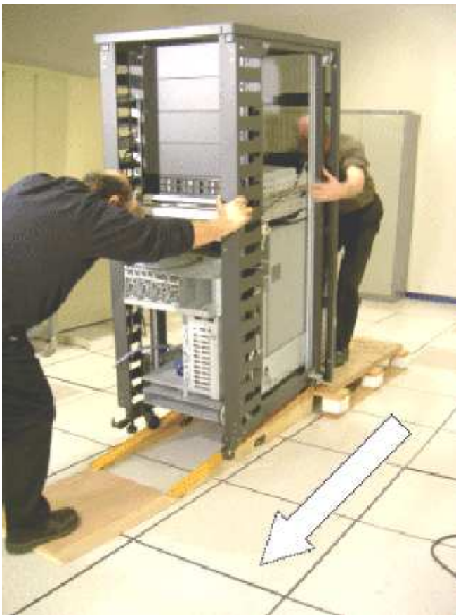
Figure 14. Unloading the 36U cabinet
