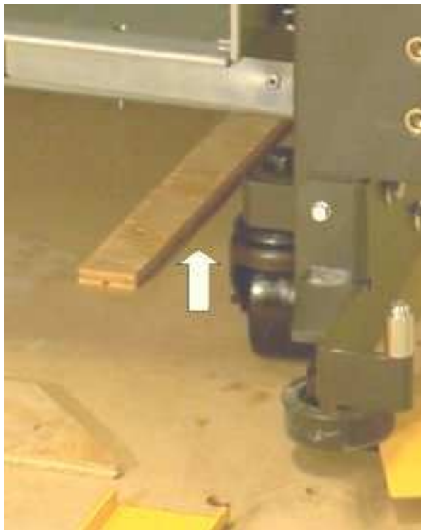
Figure 12. Positioning cabinet wheels – 36U cabinet
