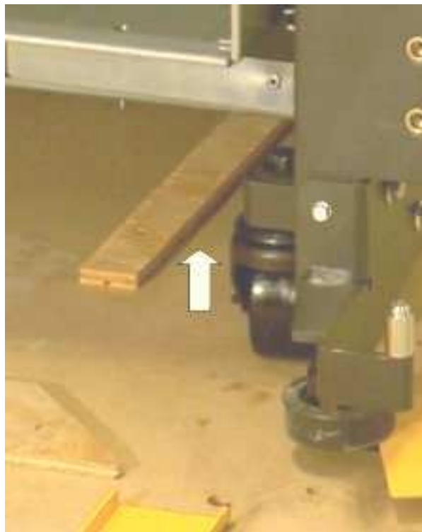
Figure 12. Positioning cabinet wheels – 36U cabinet
