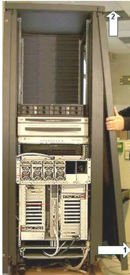
Figure 7. Removing side covers – 36U cabinet
