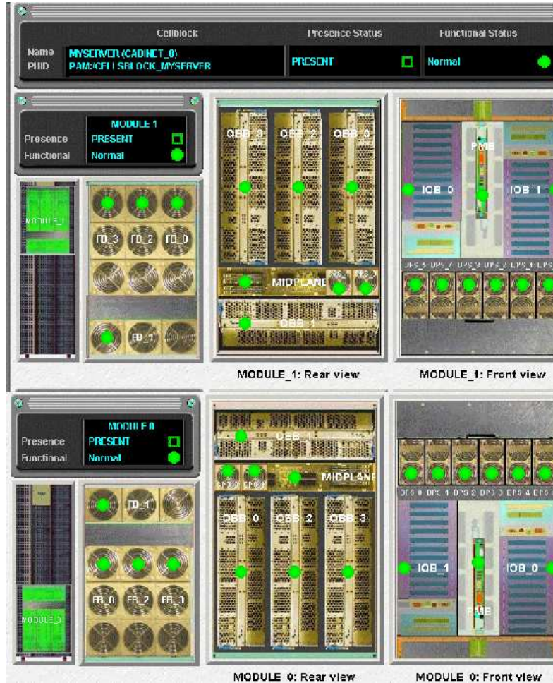
Figure 87. NovaScale 6320 Server Hardware Monitor display
