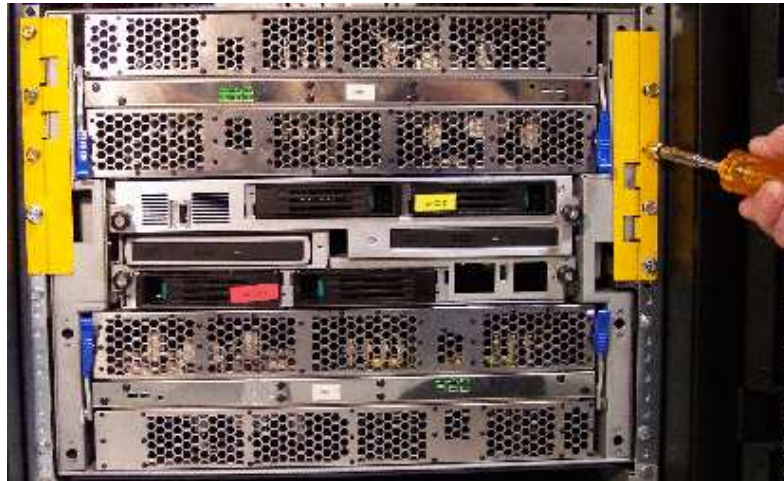
Figure 2. Removing front shipping brackets
