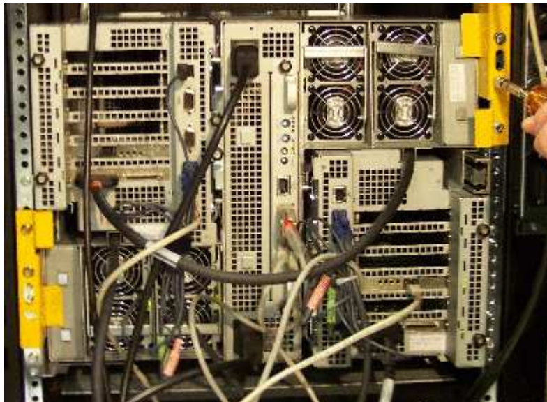
Figure 3. Removing rear shipping brackets.
