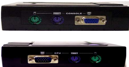
Figure 16. KVM extender (local & remote) 300m maxi.
