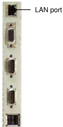
Figure 48. 10/100/1000 Mb/s LAN port
