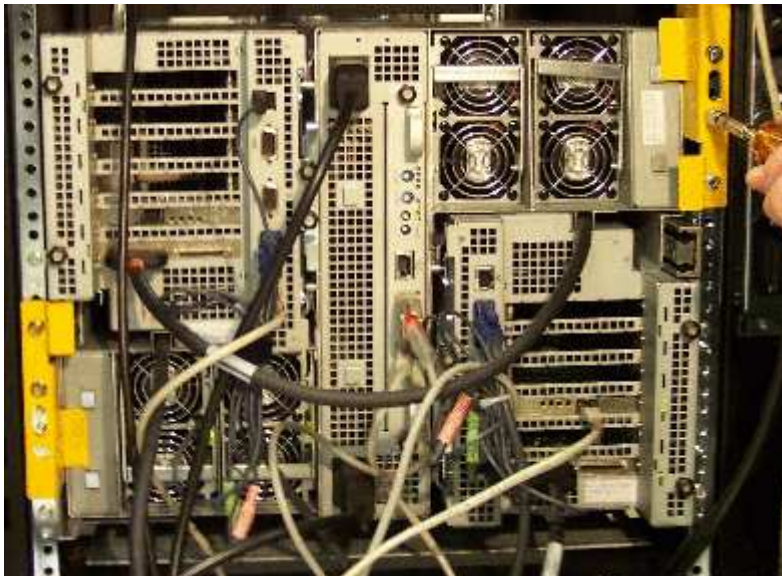
Figure 3. Removing rear shipping brackets.
