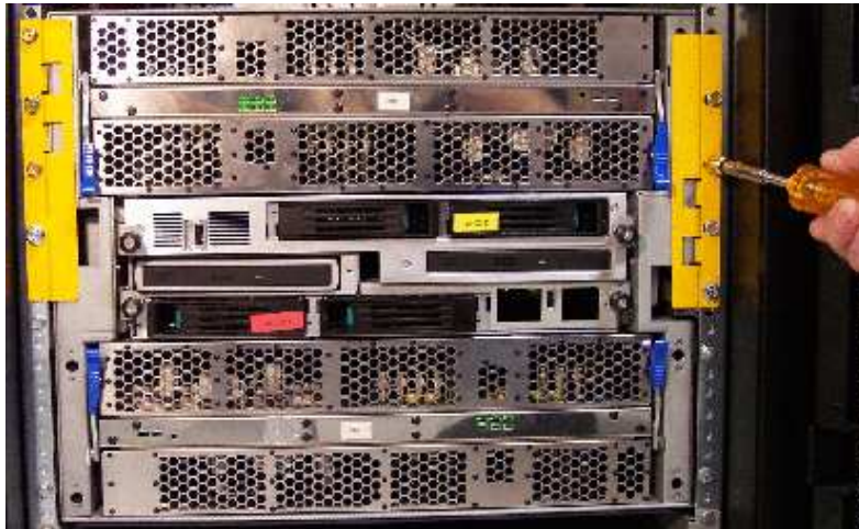
Figure 2. Removing front shipping brackets
