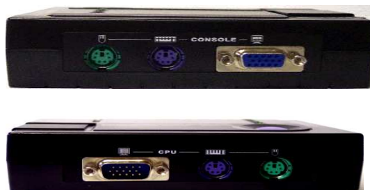
Figure 14. KVM extender (local & remote) 300m maxi.
