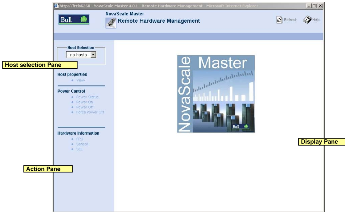
Figure 2-20 Remote Hardware Management window
