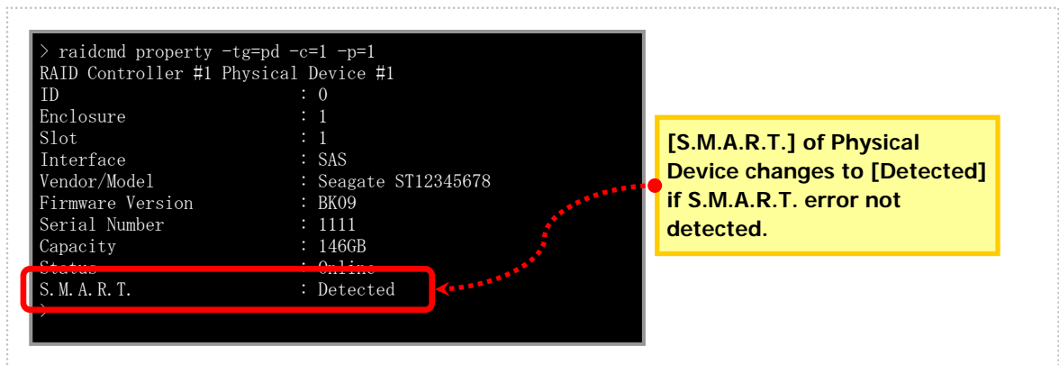
Figure 40 Display of raidcmd in detection of S.M.A.R.T. error
