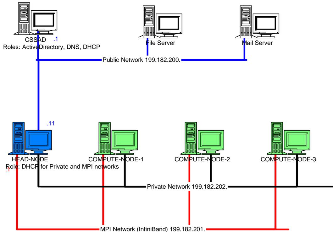
Figure 2-2. **Network Topology B** - Compute nodes isolated on private and MPI networks
