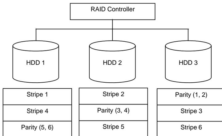
Figure 36: Configuration RAID5
