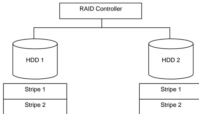
Figure 35: Configuration RAID1
