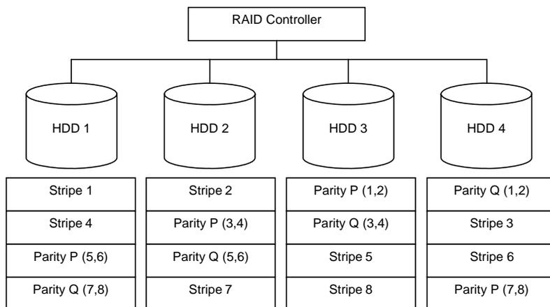
Figure 37: Configuration RAID6
