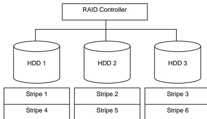
Figure 34: Configuration RAID0
