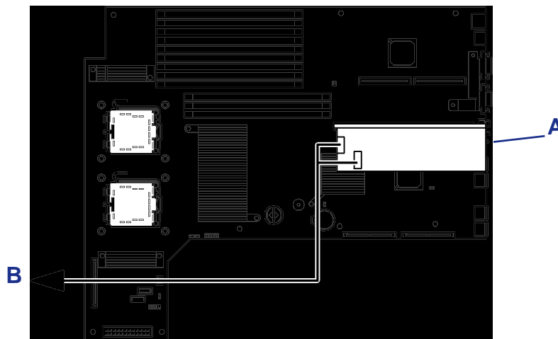
Figure 80: Rerouting the Cable Connection
