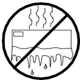
Check the system for condensation. If condensation exists, allow it to evaporate before powering on the system.
