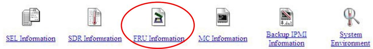
Click "FRU Information" to load Field Replaceable Unit information via the BMC. The Field Replaceable Unit (FRU) window will appear as follows:
