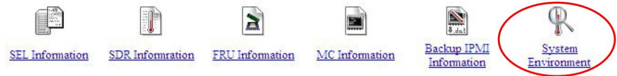
Click "System Environment" to retrieve the system environment status (temperature, voltage, fan, power, power supply unit, HDD) from the BMC and to display items (temperature, voltage, fan, power, power supply unit, HDD) of the status. The System Environment window will appear as follows:
