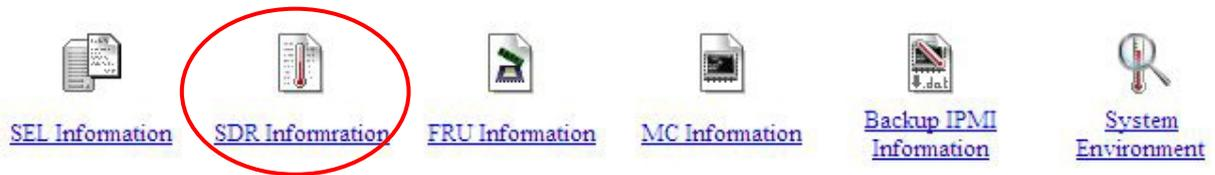
Click "SDR Information" to load sensor data records via the BMC. The Sensor Data Record (SDR) window will appear as follows:
