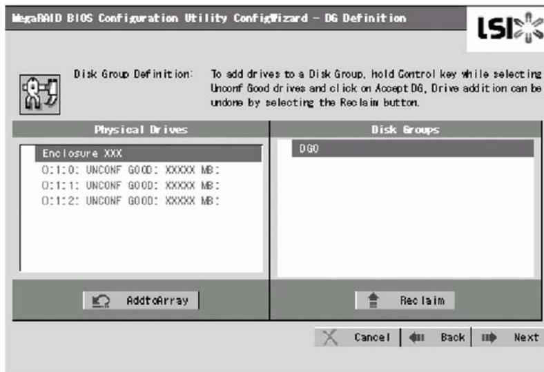
1. To add physical drives (HDDs) to a Disk Group, hold **Ctrl** and select the relevant physical drives (HDDs).
