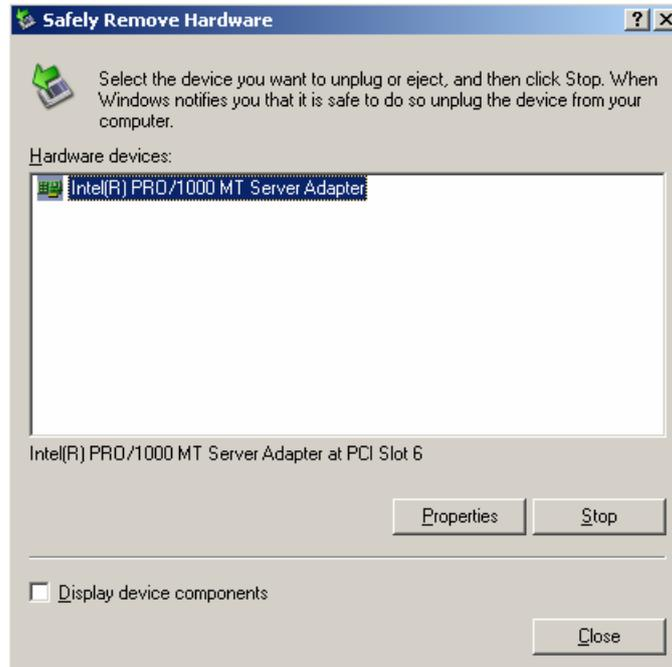
\*The message in "Hardware devices:" depends on the location of the PCI board slot and of the number of PCI boards installed.
