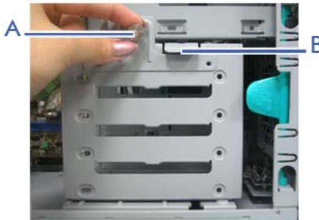
Figure 30: HDD Bracket Screw and Latch
