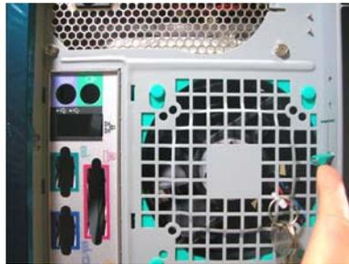
Figure 24: Right Side Door Release Latch
