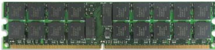
*Figure 38: DDR2 Memory Module Sample*
