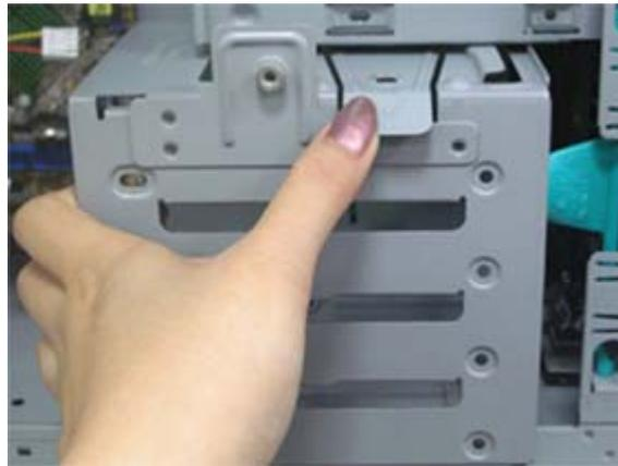
*Figure 29: Sliding the HDD Bracket out*
