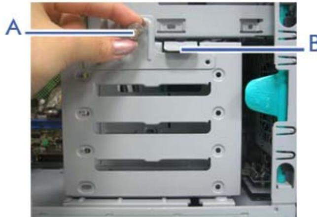
*Figure 28: HDD Bracket Screw and Latch*
