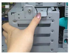
Figure 29: Sliding the HDD Bracket out
