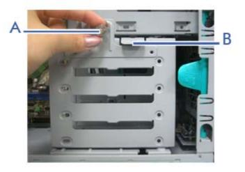
Figure 30: HDD Bracket Screw and Latch
