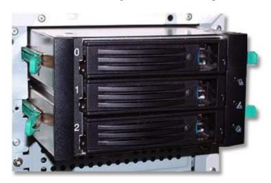
Figure 32: Installing the Hard Disk Drive Cage
