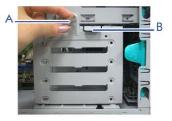
Figure 28: HDD Bracket Screw and Latch
