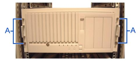
Figure 22: Securing the server to the rack cabinet
