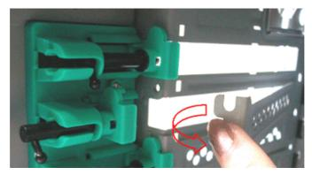
Figure 40: Removing the Expansion Slot Cover
