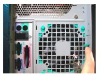
Figure 24: Right Side Door Release Latch
