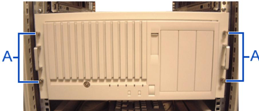
*Figure 22: Securing the server to the rack cabinet*
