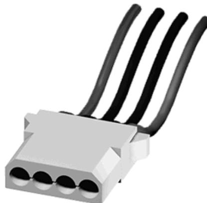
*Figure 91: IDE Storage Device Power Cable Connector*
