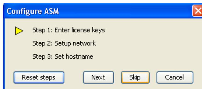
The license is already handles by the communication with the StoreWay DPA. Network parameters and host name are automatically recognized via the StoreWay DPA and all you need to do here is click three times on the button **Skip**.
